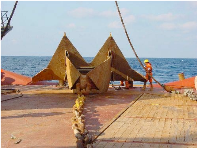
Anchor prepared for lowering
