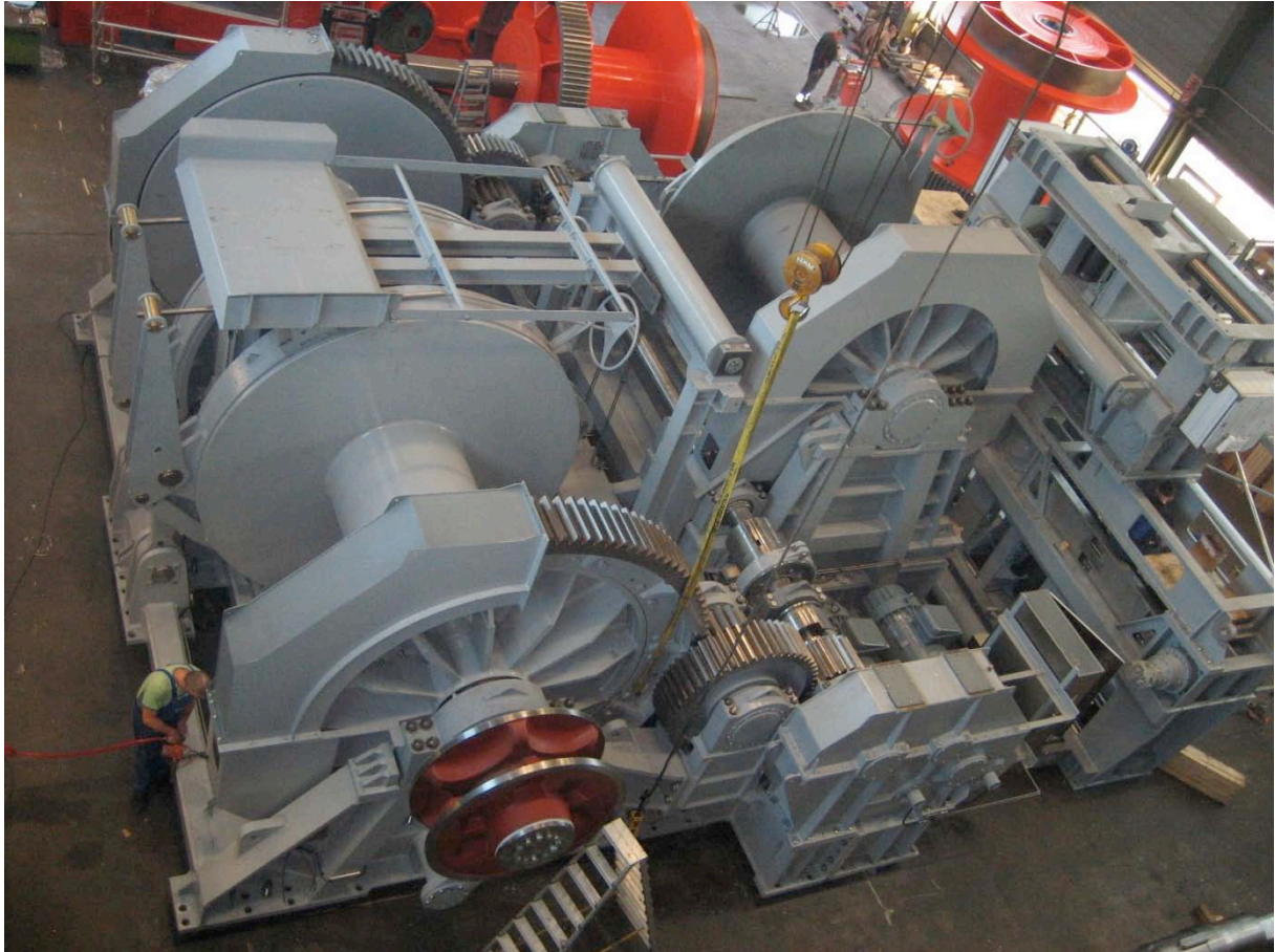
500 tons ECO-Pull winch during assembly at HATLAPA
