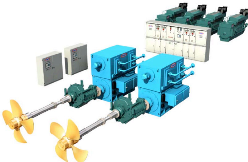
Diesel-electric concept (Source:Stadt Power Technology)
